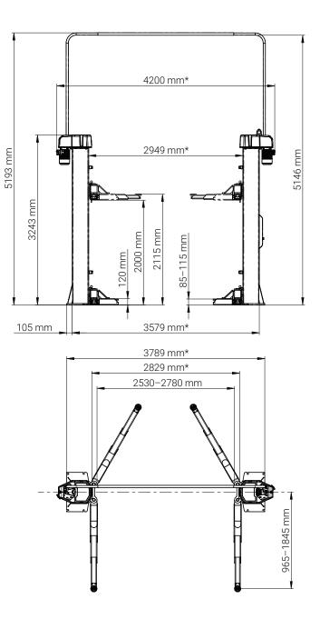
\*Dimensions refer to drive-through width of 2630 mm
