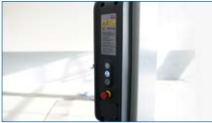
Second control unit on opposite column means less walking around the lift.
