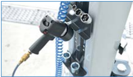
Impact wrench holder with integrated tray for support disc raisers.
